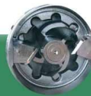
Impeller type 2 hardfacing with Widia tear edge
